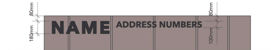
3 ADDRESS SIGN DETAIL Scale: 1:10
