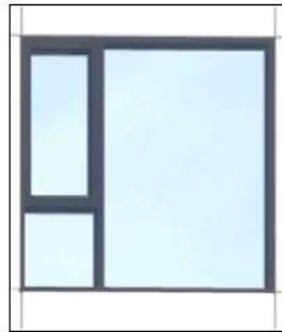
7 - Double Glazed Windows Color to Match: Benjamin Moore Black Ink 2127-20 Glass: Clear
