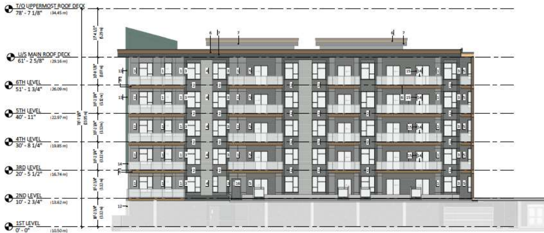
elevation - west courtyard 3/32" = 1'-0"
