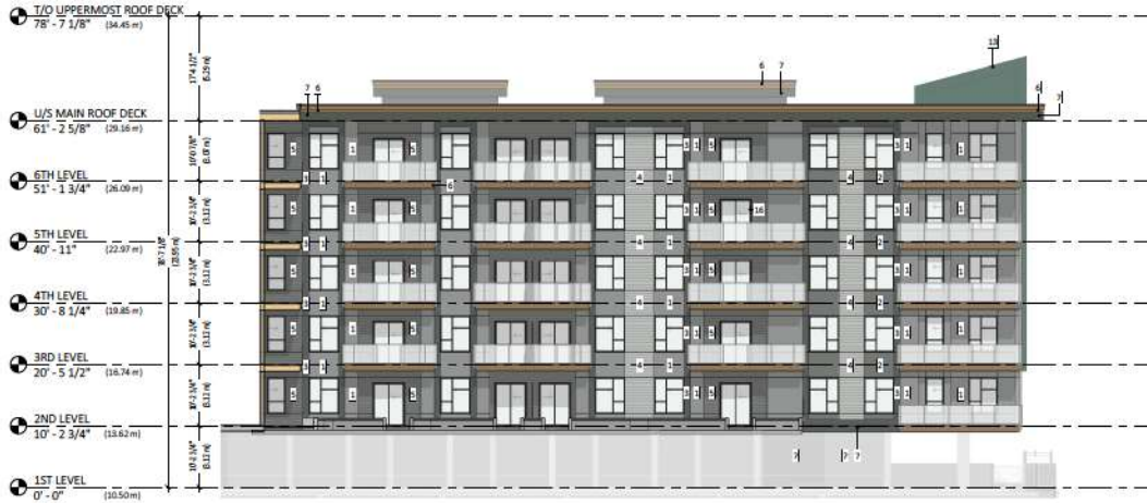
elevation - east courtyard 3/32" = 1'-0"
