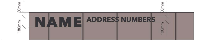
4 ADDRESS SIGN DETAIL Scale: 1:10
