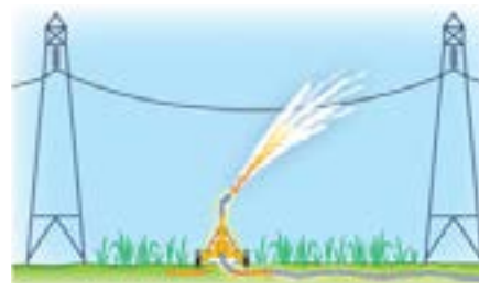
An unsafe high-angle irrigation equipment that sprays water on or near the live wires.
